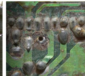
Failures on unprotected electronics
