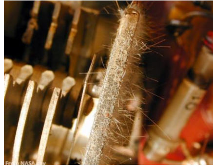
Tin whiskers Courtesy of Caplinq: link here
