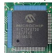
Apply dispensing/jetting lines on 2 sides of the component
