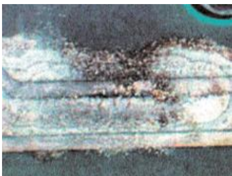
Corrosion on metal conductor
