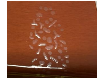
Poor adhesion due to contamination
