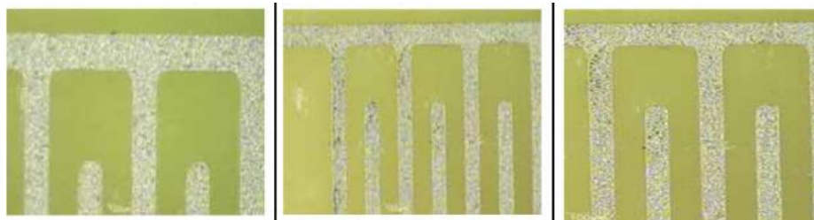
UV curable coating on test panel with Silver finish
