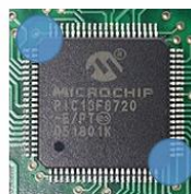
Apply dots/spots on Two of the corners
