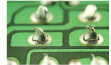
Vibration → micro-cracks and fatigue
