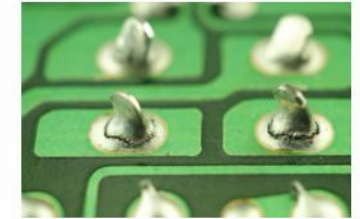
Vibration → micro-cracks and fatigue
