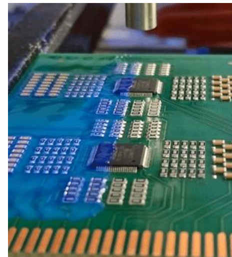
Coating application. Selective spray method
