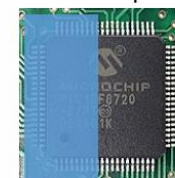
Apply coating line on half of the component
