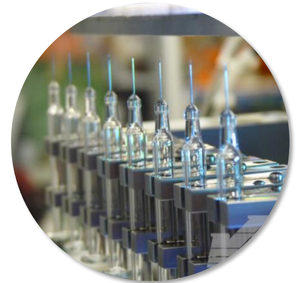
line evaluation, glass syringes traveling under a single light bar
